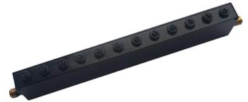
The product name of this Ocean Bandstop Filters (OBR) is OBR-5200-100, its Stop Band Frequency is 5.15-5.25GHz, Stop Band attenuation is 45dB , its Pass Band Frequency is DC-5.125GHz & 5.275-8GHz, and its Pass Band Insertion Loss is 4.0dB. Its Pass Band VSWR is 1.7.
