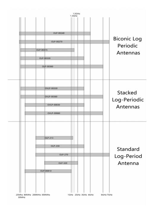
Our Log periodic antennas are divided into three different types; Standard, Stacked and Biconic Log periodic antenna. Each have different design and specific applications.
